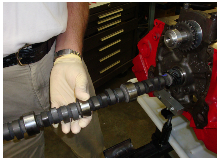
figure 3 - Clean and Dry Camshaft Installed into Bore
